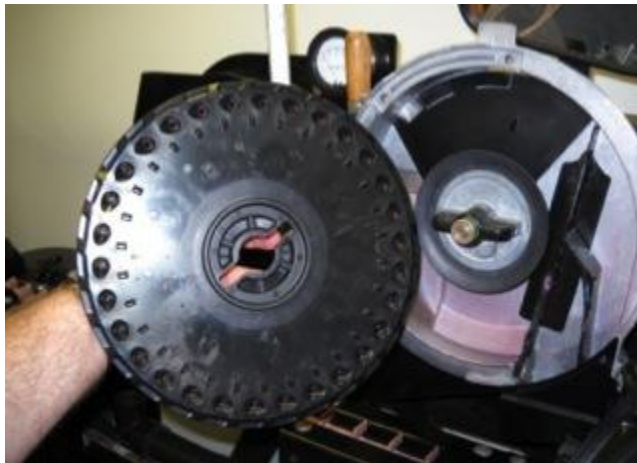
Front of Disk and Seed Chamber
